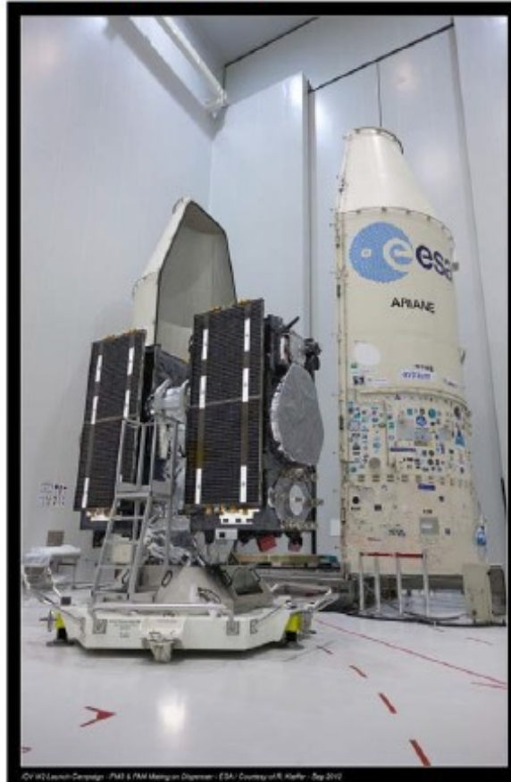
OV 02 Launch Campaign - FM3 & FM4 Mating on Dispenser - ESA - Courtesy of R. Kiefer - Sep 2012
