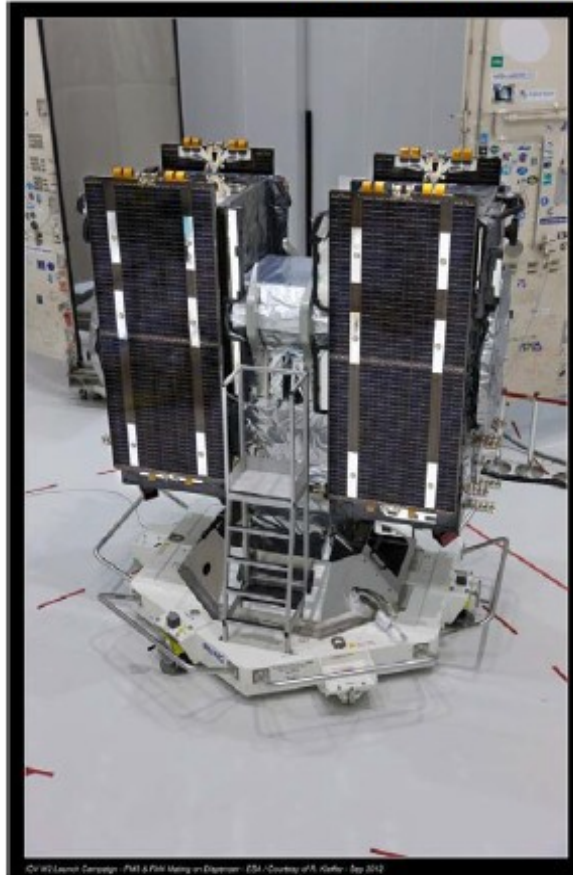
OV 02 Launch Campaign - FM3 & FM4 Mating on Dispenser - ESA - Courtesy of R. Kiefer - Sep 2012
